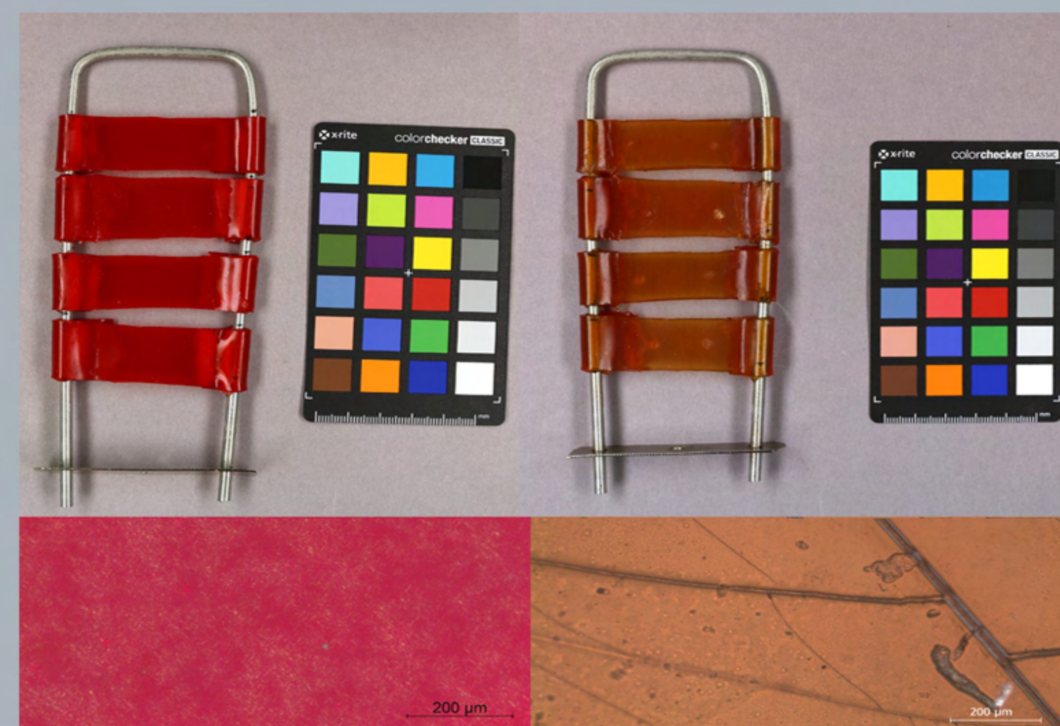
Specimen L5 before (left) and after (right) artificial light-aging
